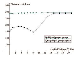
Fig. 2. I-V characteristic of the photodiode connected to a stabilized and unstabilized power source
