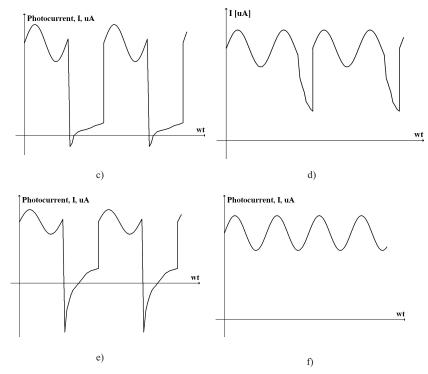
Fig. 4. Waveform of photocurrent for different voltage RMS (a) V = (0-5)V; (b) V = 6V; (c) V = 8V; (d) V = 11V; (e) V = 13V; (f) V = 15V
