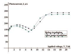
Fig. 5. I-V characteristics of photodiodes before and after irradiation
