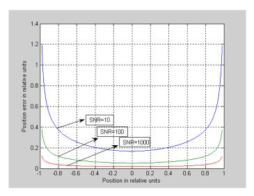
Fig. 8. Normalized position error as function normalized position for  $P_p$ =0.5, and SNR=10, 100 and 100
