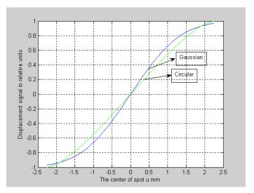
Fig. 4. Displacement signal  $\varepsilon_x$  for constant irradiance and Gaussian distribution irradiance on the surface photodiode, for r=2.1456 $\sigma$ , (r=2.25 mm,  $\sigma$ =1.048 mm)
