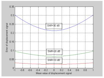
Fig. 7. The error of displacement signal as function mean value, for Pp=50% and SNR=10 dB, 20 dB, and 30 dB.
