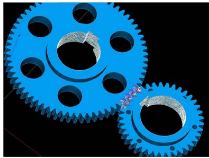
Figure 3: Displacement and force boundary conditions
